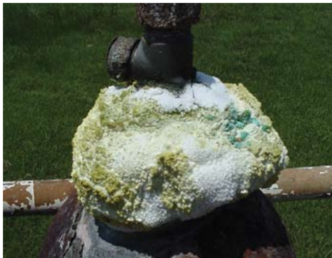
Sometimes, gas cylinders are improperly stored and corrosion can leave them extremely unstable.
