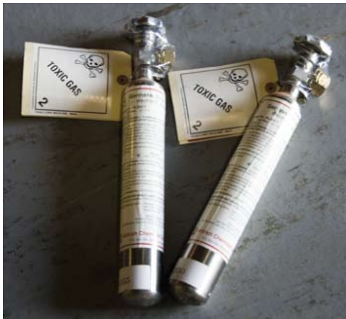
Elbow bottles such as those shown above are used in many situations but are often not well marked as to content.
