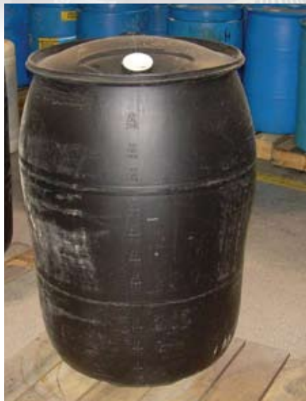
The above drum is bulging. It must be handled with extreme care to avoid a major mishap.
